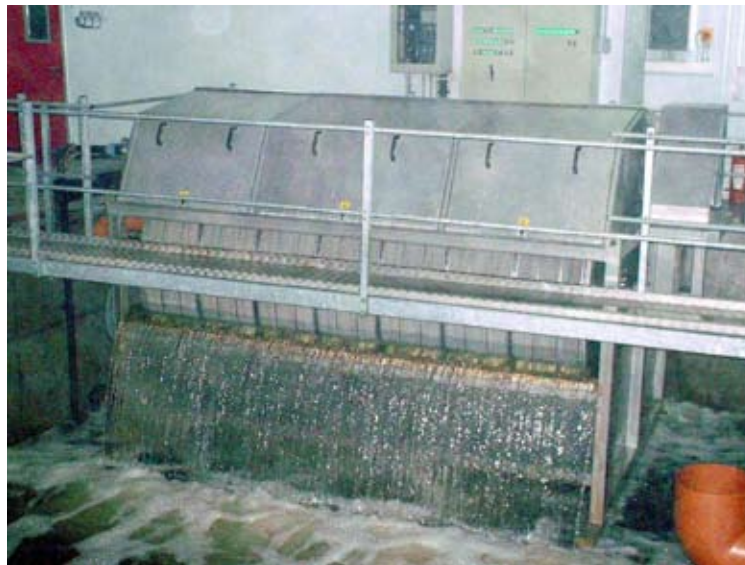
Drumfilter model HDF2007-1A in a recirculated salmon farm
